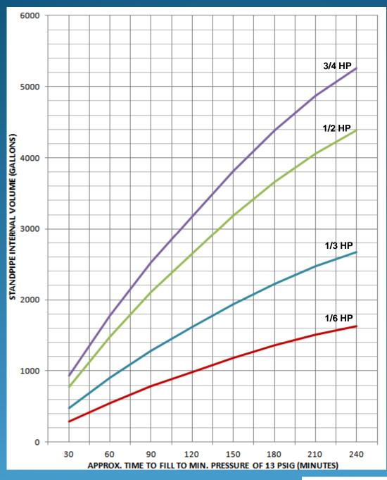
Fill time is important for estimating downtime when standpipe is added to or sections are removed. A quicker fill time allows the standpipe to be returned to service sooner. Boston FD TCM3-51725 mandates ceasing all construction or demolition operations if the standpipe is not restored within 4 hours of impairment. Choose compressor size accordingly.
