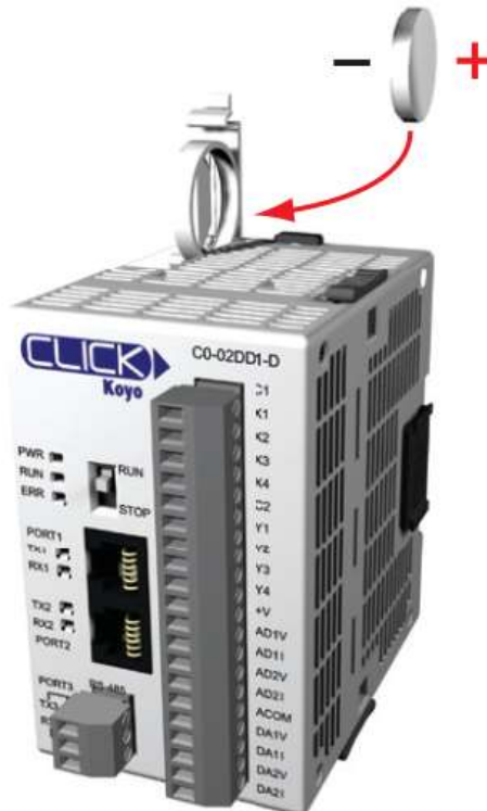
Figure 25 Replacement of PLC Backup Battery
