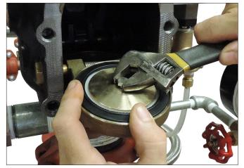
**11.** Tighten the seal assembly bolt/bolt seal to the torque value listed in the table on this page to ensure a proper seal.
