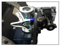
5. Crimp a spade connector onto NEUTRAL wire.
