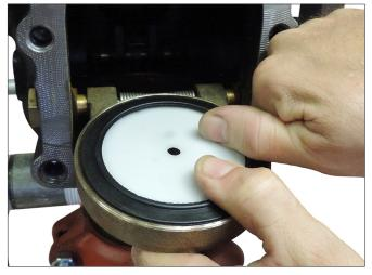
**9.** Install the clapper seal into the clapper carefully. Ensure that the seal ring snaps into the clapper completely.
