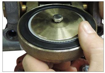
**10.** Place the seal-retaining ring onto the seal washer of the clapper seal. Install the seal assembly bolt/bolt seal through the seal-retaining ring and clapper.
