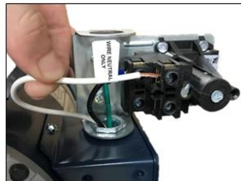
4. Remove yellow wire nut from motor NEUTRAL.
