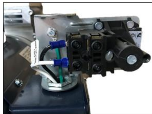
6. Insert spade connector into other motor terminal. Use wiring diagram on side of motor to wire it for 230V. 7. Wire supply line 1 and line 2 to line contacts of pressure switch.
