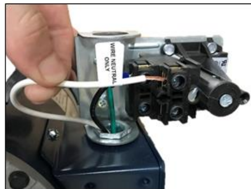
4. Remove yellow wire nut from motor NEUTRAL.
