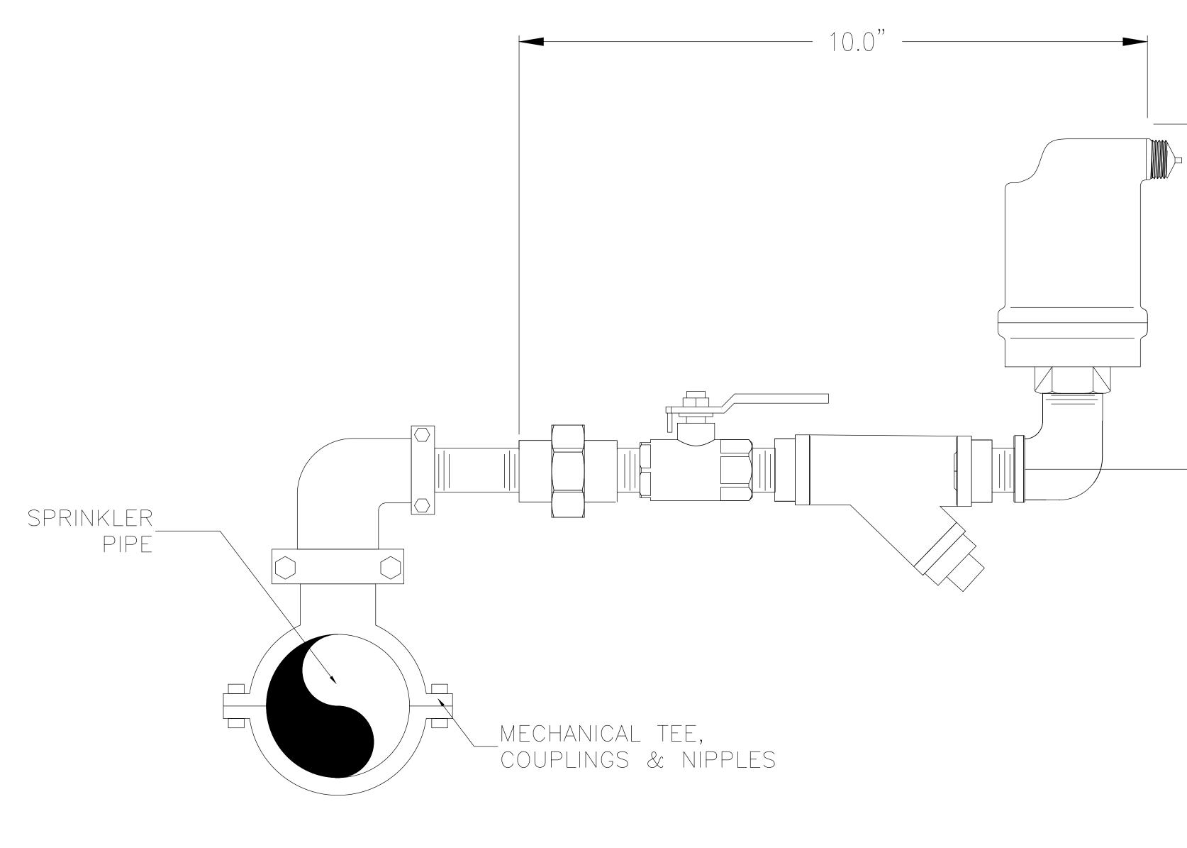
**DIMENSIONS AND INSTALLATION** MODEL AR-1 WET SPRINKLER AIR VENT
