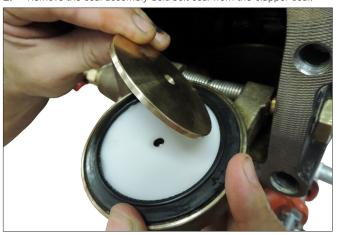
Remove the seal-retaining ring. Save the seal-retaining ring for re-installation.
