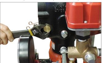
Remove the clapper shaft bushings with o-rings from the valve body.
