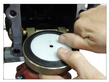
9. Install the clapper seal into the clapper carefully. Verify that the seal ring snaps into the clapper completely.
