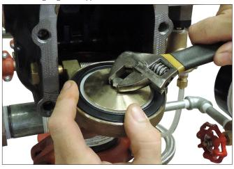
**11.** Tighten the seal assembly bolt/bolt seal to the torque value listed in the table on this page to ensure a proper seal.
