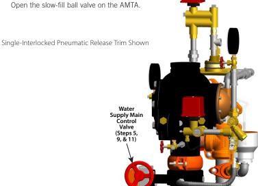
8. Open the water supply main drain valve (lower drain valve).
