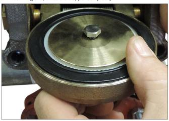
Place the seal-retaining ring onto the seal washer of the clapper seal. Install the seal assembly bolt/bolt seal through the sealretaining ring and clapper.
